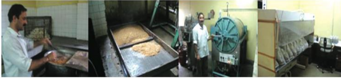
(a) Boiling, sieving, autoclaving and inoculation
