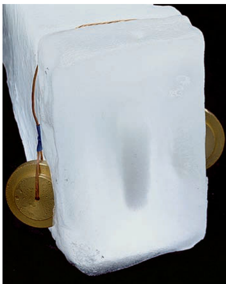
Figure 10.30 Pressure and melting point. Why does the weighted wire cut through this block of ice?
