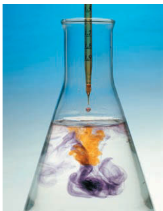
▲ The reddish \text{I}_3^- solution turns a deep blue color when it is added to a solution containing a small amount of starch.
