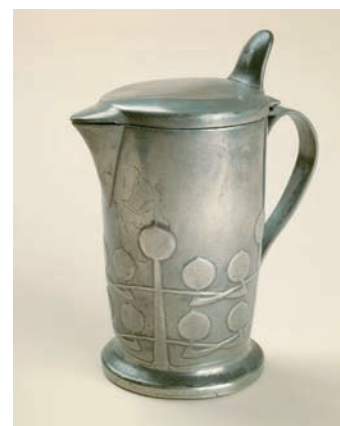
▲ The pewter in this 200 year old jug is a solid/solid solution of approximately 96% tin and 4% copper.
