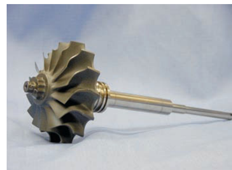
▲ A silicon nitride rotor for use in gas-turbine engines.
