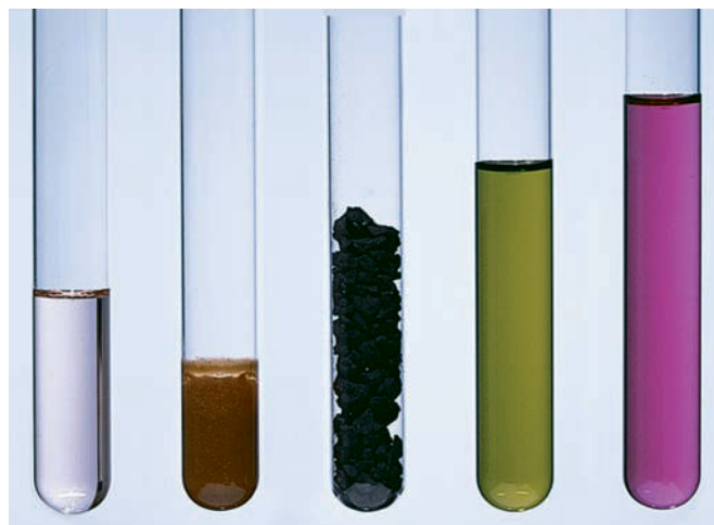
Manganese species: \text{Mn}^{2+}(aq) \text{Mn}(\text{OH})_3(s) \text{MnO}_2(s) \text{MnO}_4^{2-}(aq) \text{MnO}_4^{-}(aq) Oxidation state of manganese: +2 +3 +4 +6 +7
