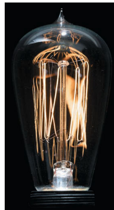
Figure 21.4 The incandescent lightbulb. The bulb emits white light when an electric current passes through the tungsten wire filament, heating it to a high temperature. The glass bulb contains gases such as argon and nitrogen, which carry away heat from the filament. Although tungsten has the highest boiling point of any element (5555 °C), the tungsten slowly evaporates from the hot filament and condenses as the black spot of tungsten metal usually visible on the inside surface of a burned-out bulb.
