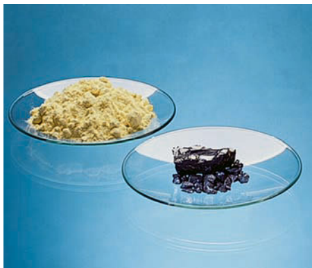
▲ These samples of sulfur and carbon have different masses but contain the same number of atoms.
