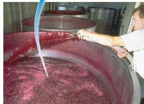
▲ Fermentation of the sugar from grapes yields the ethyl alcohol in wine.
