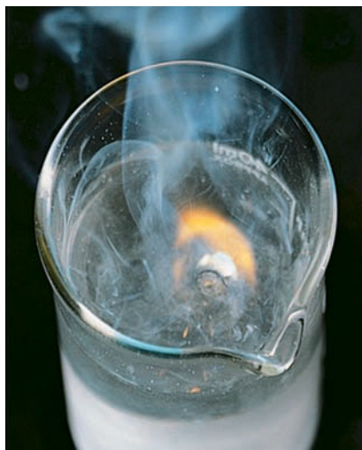
▲ Sodium, one of the alkali metals, reacts violently with water to yield hydrogen gas and an alkaline (basic) solution.
