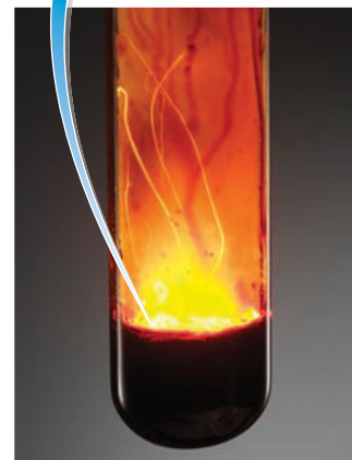
▲ Aluminum metal reacts with liquid bromine in a spectacular display of sparks.
