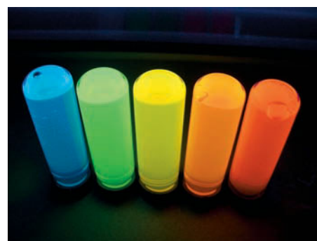
▲ The color of these semiconductor nanoparticles, called quantum dots, varies from red to violet as the size of the nanoparticles decreases.
