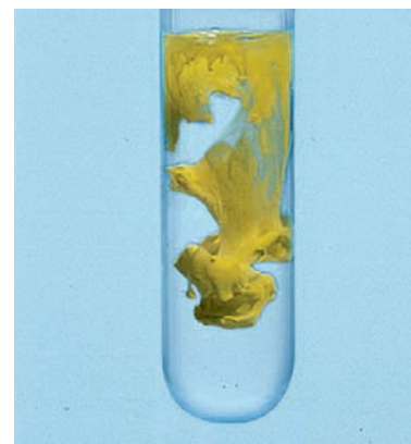
▲ Reaction of aqueous \text{Pb}(\text{NO}_3)_2 with aqueous \text{KI} gives a yellow precipitate of \text{PbI}_2 .
