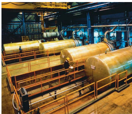
▲ Much of the uranium-235 used as a fuel in nuclear reactors is obtained by gas diffusion of \text{UF}_6 in these cylinders.
