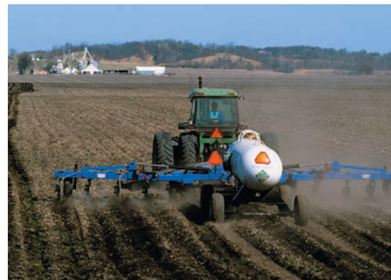
▲ Ammonia is injected directly into a field from tanks containing liquid ammonia under pressure.
