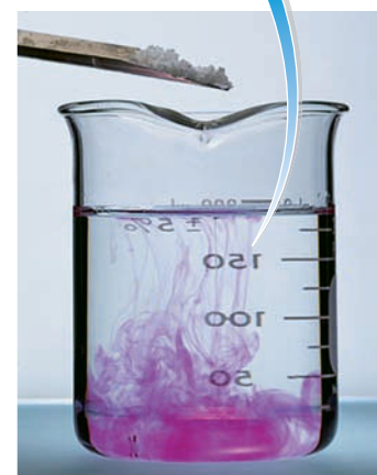
▲ Dissolution of sodium peroxide in water that contains phenolphthalein gives a red color due to formation of OH - ions.
