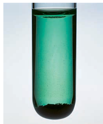
▲ Adding H_2S to an acidic solution of Hg^{2+} and Ni^{2+} precipitates Hg^{2+} as black HgS but leaves green Ni^{2+} in solution.
