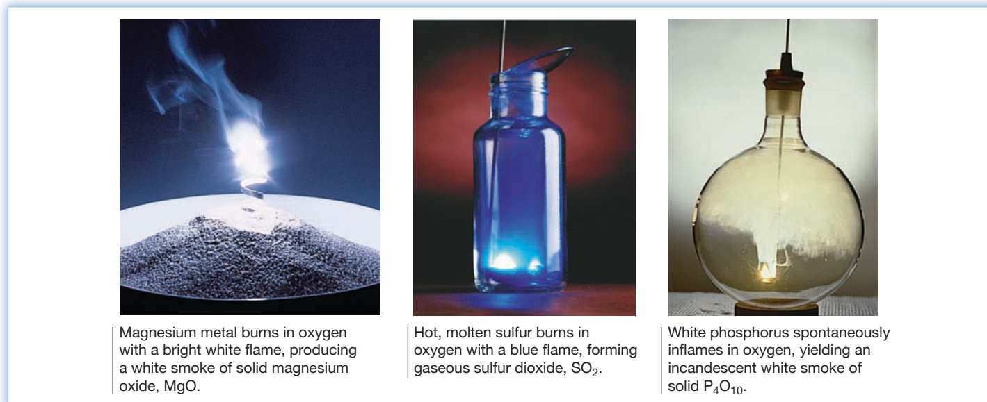
Figure 18.5 Some reactions of oxygen.
