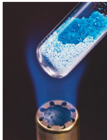
Figure 18.11 Blue crystals of \text{CuSO}_4 \cdot 5 \text{H}_2\text{O} are converted to white anhydrous \text{CuSO}_4 when the sample is heated with a Bunsen flame.
