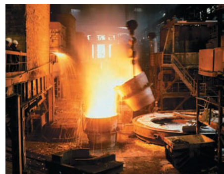
▲ Crude iron is converted to steel by oxidizing impurities with \text{O}_2 gas.
