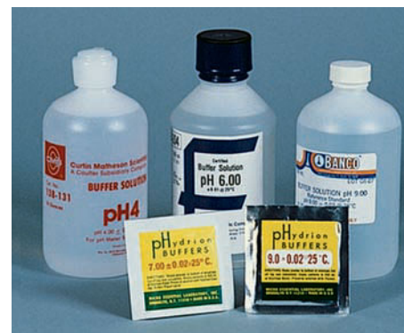
Figure 15.5 Prepackaged buffer solutions of known pH and solid ingredients for preparing buffer solutions of known pH.
