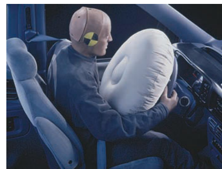
▲ Automobile air bags are inflated with \text{N}_2 gas produced by decomposition of sodium azide.
