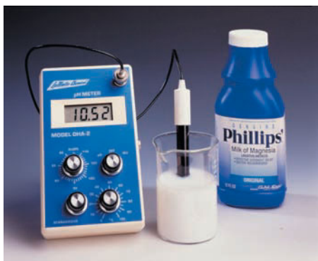
Figure 14.5 A pH meter with its electrical probe dipping into milk of magnesia. An accurate value of the pH (10.52) is shown on the meter.
