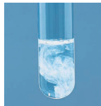
▲ Addition of a solution of silver nitrate to a solution of sodium chloride yields a white precipitate of solid silver chloride.
