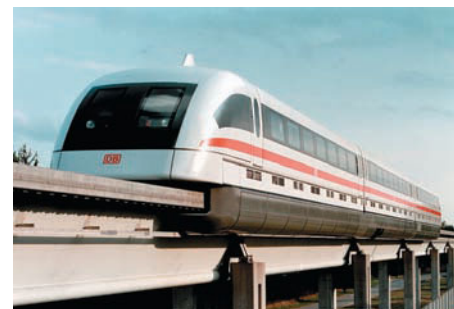
Figure 21.19 A Maglev train is now in commercial operation in Shanghai, China, running at 430 km/h.
